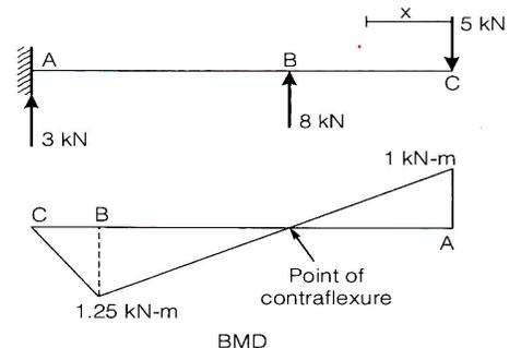
Distance of point of contraflexure from A is  $x$ ,  $5(1-x) - 8(0.75-x) = 0$
