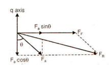
In this case the armature reaction is partially magnetising due to F<sub>s</sub>sinθ component and partially magnetising due to  $F_c \cos\theta$  component
