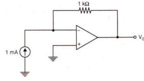
$$0 - V_o = 1 \text{ mA} \times 1 \text{k}\Omega$$
