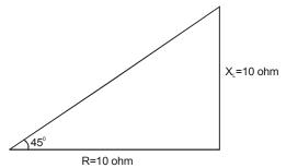
Hence the phase angle between voltage and current =  $45^{\circ}$
