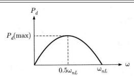
Developed power will be maximum at a speed equals to  $0.5 \text{ w}_{ml}$ .
