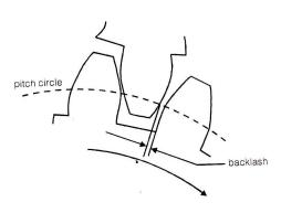
Backlash is defined as the amount by which the width of tooth space exceeds the thickness of the engagement tooth measured along the pitch circle.
